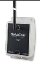
The RQT offers the same wireless alerting features and battery powered operation as the RQA, with the exception that the RQT package is mounted inside the custom kiosk and is hidden from view. The retailer supplied Call Button, attached to the kiosk, is then remotely hardwired to the RQT. Only the customer service Call Button is visible to the shopper.
